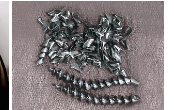
Long chip and center wear noted
